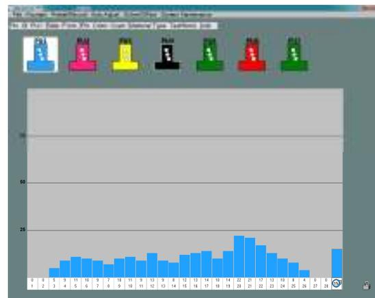
**AutoSet** can be configured to automatically process files from the CTP or Image Setter work flow and transfer the presetting data to the Ink Desk
